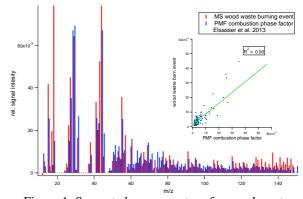
Figure 1. Separated mass spectra of a wood waste burning event measured by the ACSM at the Hohenpeißenberg site in 2015, which is compared with a PMF factor of the combustion phase during a wood combustion experiment in a logwood stove measured by an aerosol mass spectrometer.
